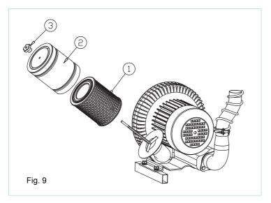
After approx. 20 hours of operation the air filter (fig. 9-1) should be cleaned.
